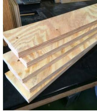
Fig. 2. Angle-ply wood laminate torsion test specimens fabricated and tested at UMass in 2014
